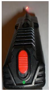
[H] Showing Enforcer is on (Safety-up) and battery is charge and ready for download.
