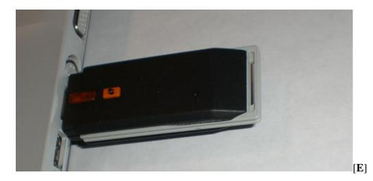
**4:** Now <u>plug-in</u> USB data port reader TC-100. Wait about thirty-seconds for drivers to find data port and load. You should see at bottom right "Windows looking, finding and acknowledging install is complete". If not, un-plug USB data port reader and reinstall once again. If Windows Operating System still cannot find data port reader, then find another USB port to plug-in and operate from.
