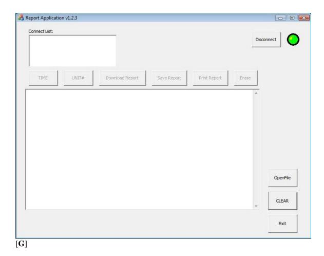
**8:** Turn on PhaZZer Enforcer and wait five-seconds for data port reader to communicate with Enforcer and show ID number of Enforcer in "Connect List" box. See [I].
