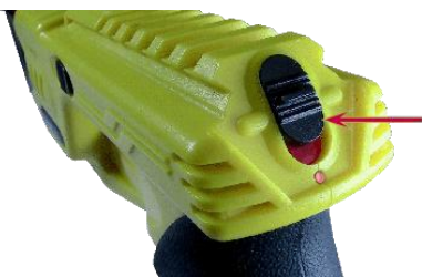
Laser & Activation Switch with LED
